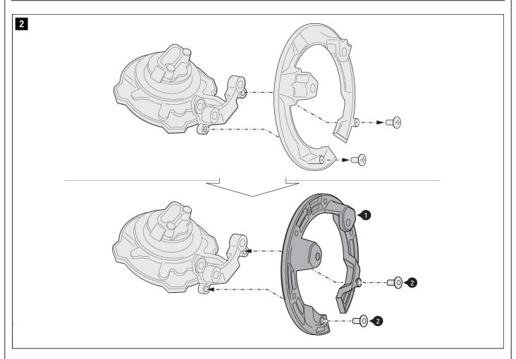
Unscrew the screws from the cap unit.
