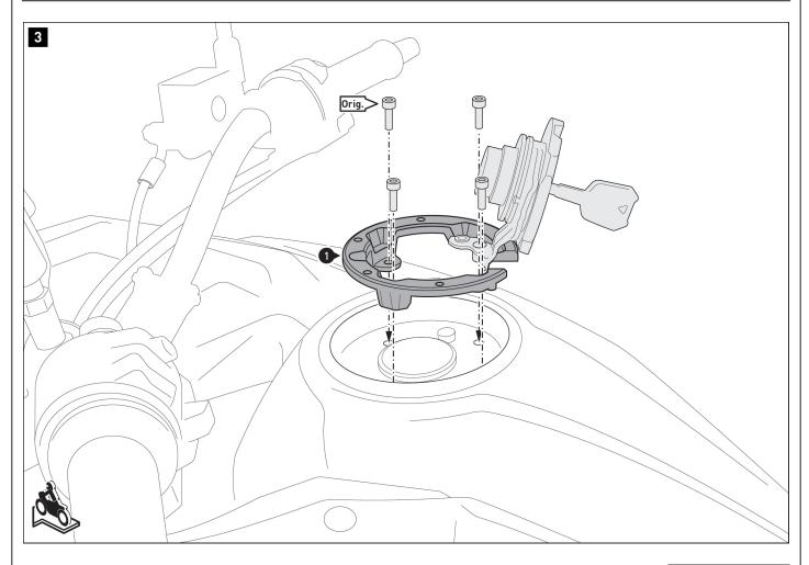
Screw the tank ring adaptor (1) onto the vehicle using the original (orig.)
