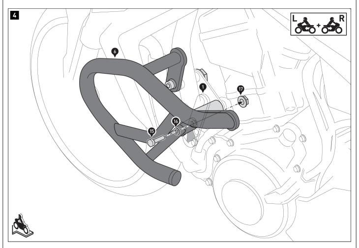
Screw the left crash bar (6) to the mounting bracket (1) and to the vehicle. When all components have been loosely attached, tighten screws (15) as specified in the mounting instructions.
