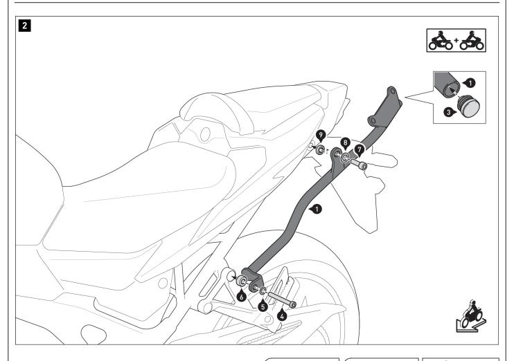
$\triangle$  **NOTE:** If the SW-MOTECH side carrier is installed at the same time, the add-on parts (4), (5), (7) and (8) are omitted. Instead of these add-on parts, mount the side carrier(s) using the enclosed add-on parts.
