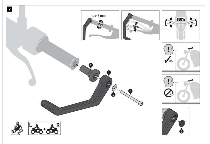
Screw the lever guards [1] to the handlebar ends on both sides. **A WARNING:** Use a liquid threadlocker!
