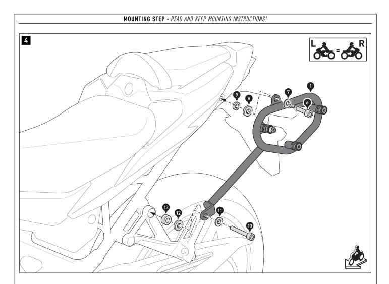
▲ **NOTICE:** If the SW-MOTECH rack (\*) is being mounted at the same time, spacers (8), (9), (12) and (13) are not to be used. Instead, use the spacers (\*) supplied with the rack.
