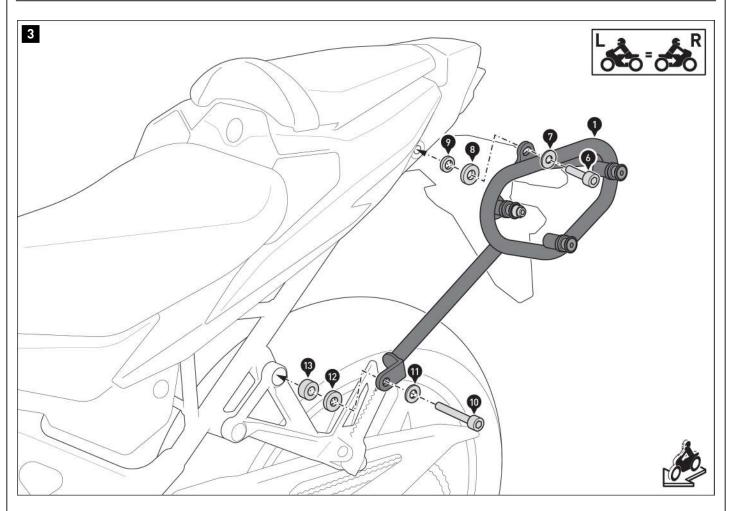
Screw the side carrier (1) to the rear of the vehicle. **AWARNING:** Use a liquid threadlocker!
