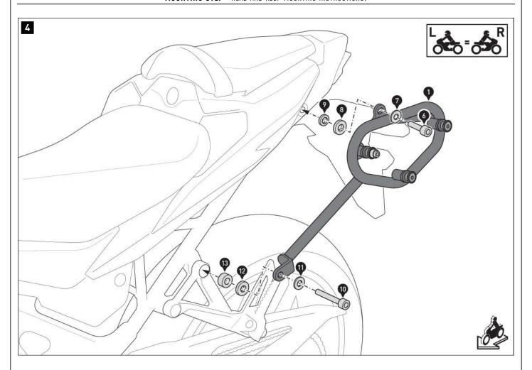
$\triangle$  **NOTICE:** If the SW-MOTECH rack (\*) is being mounted at the same time, spacers (8), (9), (12) and (13) are not to be used. Instead, use the spacers (\*) supplied with the rack.
