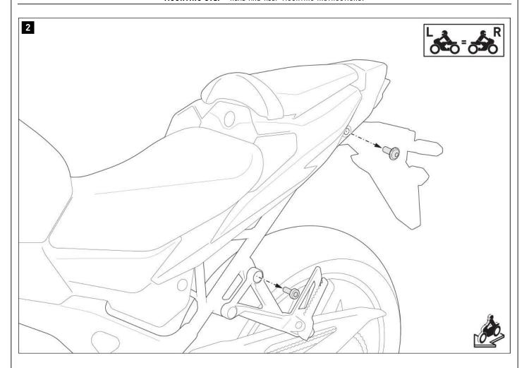
Loosen the screws from the attachment points indicated.
