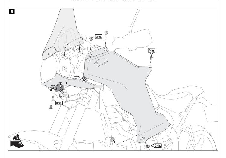
Reattach the previously disassembled trim parts to the vehicle. WARNING: use liquid thread locker! Tighten the original (Orig.) screws according to the manufacturer's instructions.
