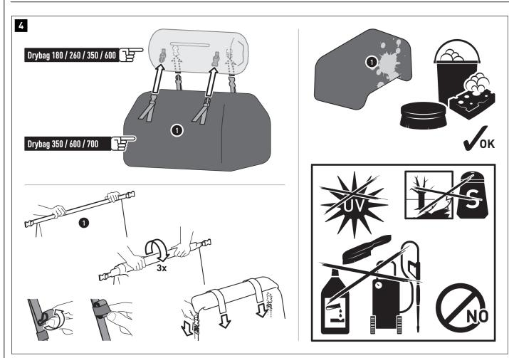
The tail bags are designed to be attached to other tail bags from the Drybag series. Connect the tail bags using the buckles **(max. TWO tail bags on top of each other per vehicle; the LOWER bag must be larger than the UPPER bag)**. Then ensure that all buckles are correctly positioned and securely held.
