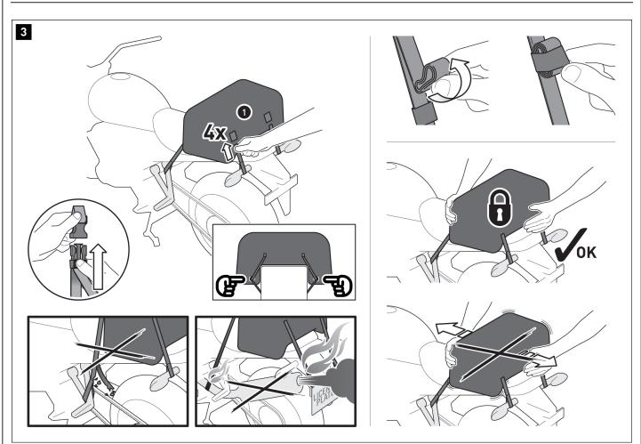
Connect the lashing straps (3) to the tail bag (1). Then tighten the lashing straps (3).
