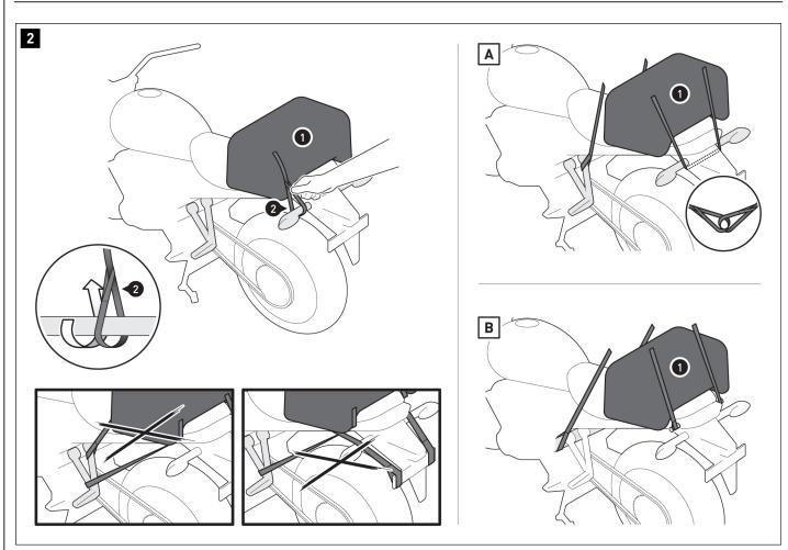
Loop the lashing straps (3) at **FOUR** suitable, sturdy attachment points on the vehicle, as shown in the drawing and examples **[A]** and **[B]** (ex. footrest mount, vehicle frame, luggage hook, etc.). Be sure to attach the appropriate lashing strap to the attachment points (male to female; female to male) for the buckles on the bag.
