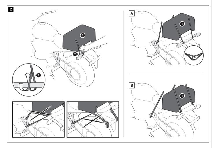
Loop the lashing straps (3) at **FOUR** suitable and resilient attachment points on the vehicle, as shown in the drawing and the example drawings**[A]** and**[B]** shown (ex. B. footrest mount, vehicle frame, luggage hook, etc.). Be sure to attach the appropriate lashing strap to the attachment points (male to female; female to male) for the buckles on the bag.
