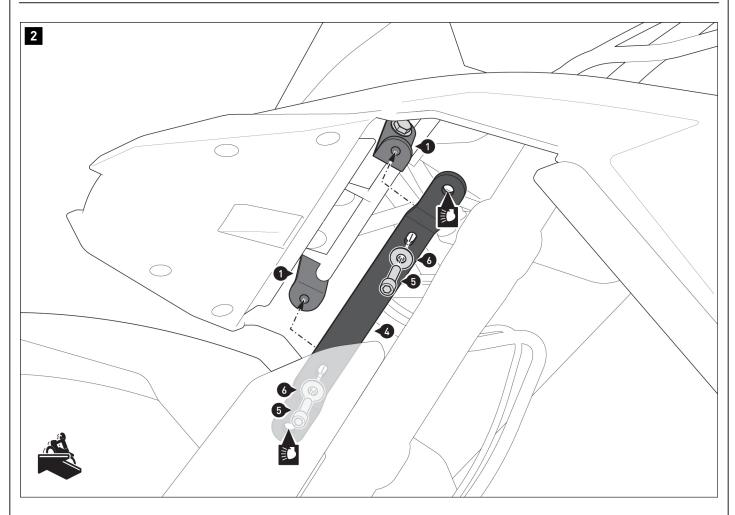
Mount the headlight holder [4] on the mounting brackets [1]. **A** WARNING: Use a liquid threadlocker!
