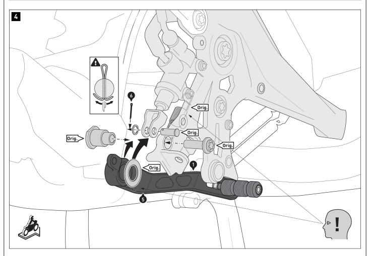
Screw the brake lever to the vehicle using the original parts (Orig.).
