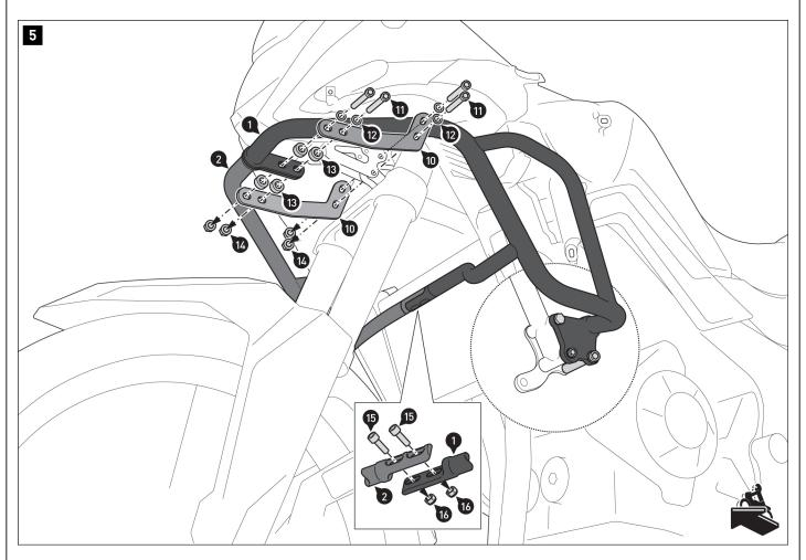
Screw the mounting brackets (10) onto the vehicle. Do not tighten the screws (11) yet.
