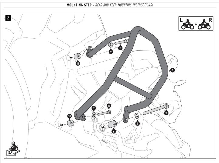
Screw the left crash bar [1] to the vehicle. **A WARNING: use liquid thread locker!** Tighten all screws according to the manufacturer's instructions.
