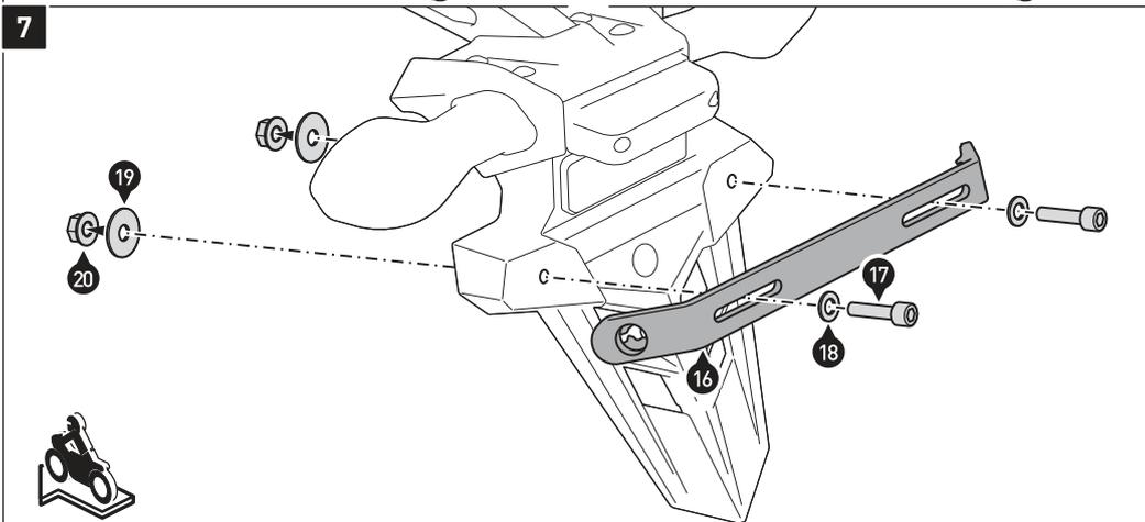
**NOTE:** Follow step [5] and [6] only if the mounting holes of the mudguard do not match with the hole pattern of the crossbar (16).
